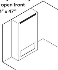
Open chase framing with enclosure min 1-1/4" below ceiling
