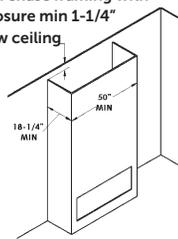
Framing to ceiling with vents at front and back
