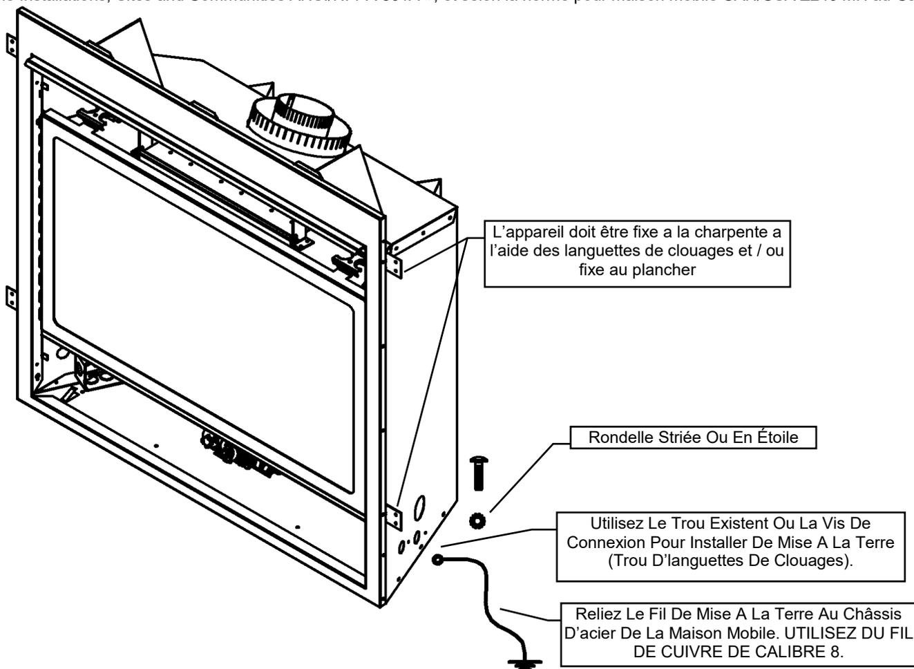
LES CHAUFFAGES À FOYER À GAZ VENTILÉ (ANSI Z21.88) DANS CE MANUEL, PEUT ÊTRE INSTALLÉ DANS FABRIQUÉS (MOBILES) LA PREMIÈRE VENTE APRÈS DANS LE ÉTATS-UNIS.
