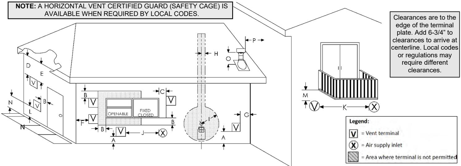
Clearances are to the edge of the terminal plate. Add 6-3/4" to clearances to arrive at centerline. Local codes or regulations may require different clearances.
