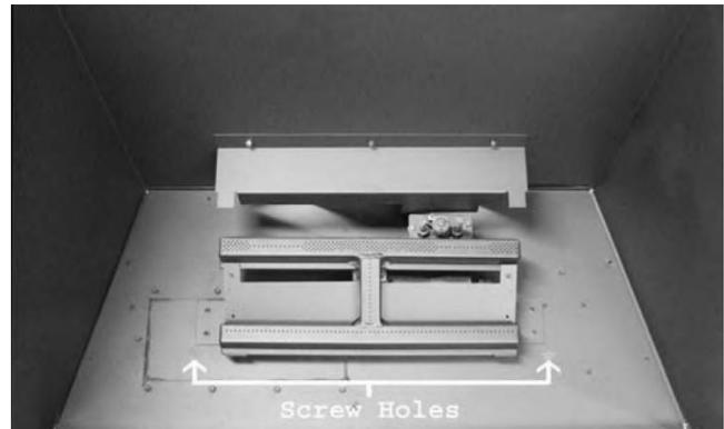
**STEP 2:** Replace/reinstall the 2 screws from the grate bar.
