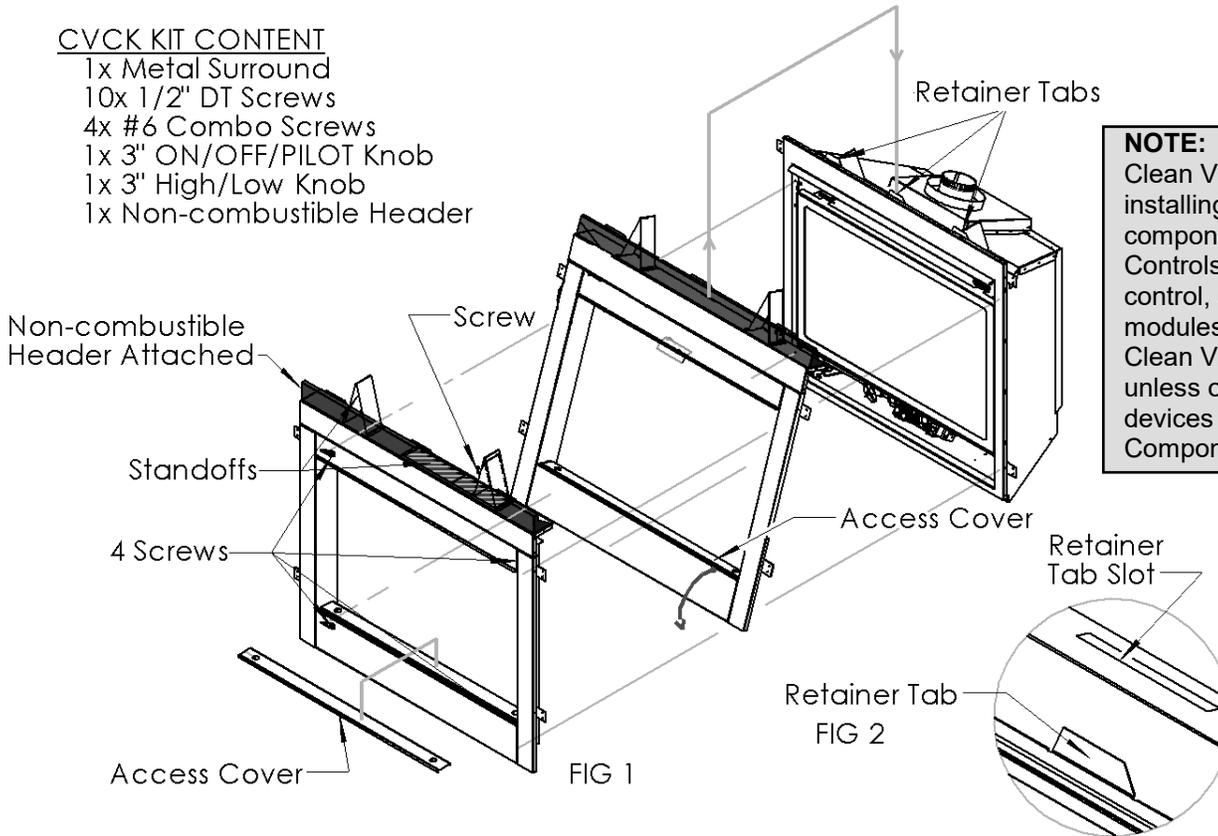
**NOTE:** When using the Clean View Kit (CVCK) and installing optional electrical components (i.e. Remote Controls, variable speed control, and or fan modules) locate them in the Clean View access area, unless other shielding devices like our IPI Component box is used.
