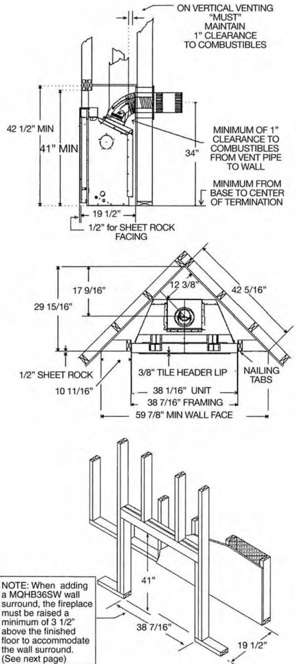
NOTE: When adding a MQHB36SW wall surround, the fireplace must be raised a minimum of 3 1/2" above the finished floor to accommodate the wall surround. (See next page)
