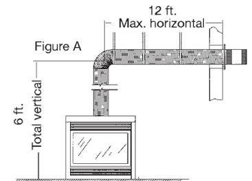
**NOTE: The final location of the fireplace must be such that the horizontal vent dimensions fall within those stated on the graph. The Maximum Vertical vent run is 40ft. (12.2 meters).**
