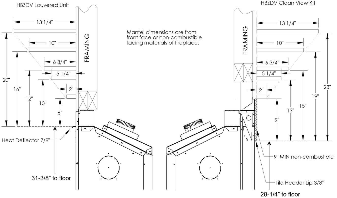
**Warning:** Combustible objects must not be placed on a non-combustible mantel unless the non-combustible mantel meets the minimum height and width requirements for a combustible mantel.
