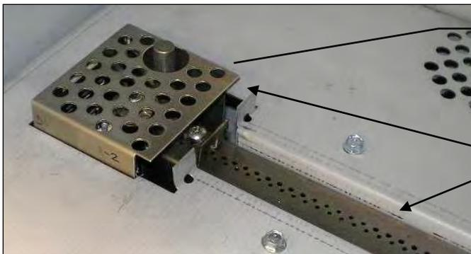
\*Pilot Shield should be visually inspected monthly for signs of deterioration due to flame exposure. Replace if necessary.
