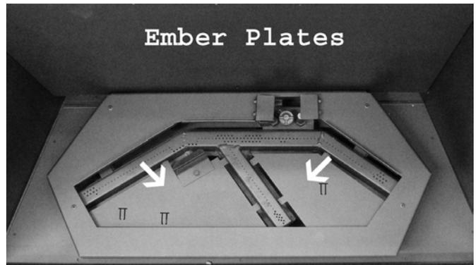
**Step 3:** Using the left ember plate mounting bracket, slide the left ember plate into position as shown. Repeat the same for the right ember plate
