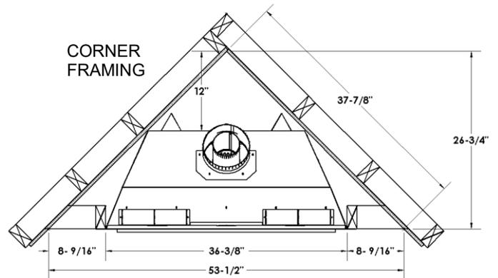
**Framing for Horizontal Vent Termination
