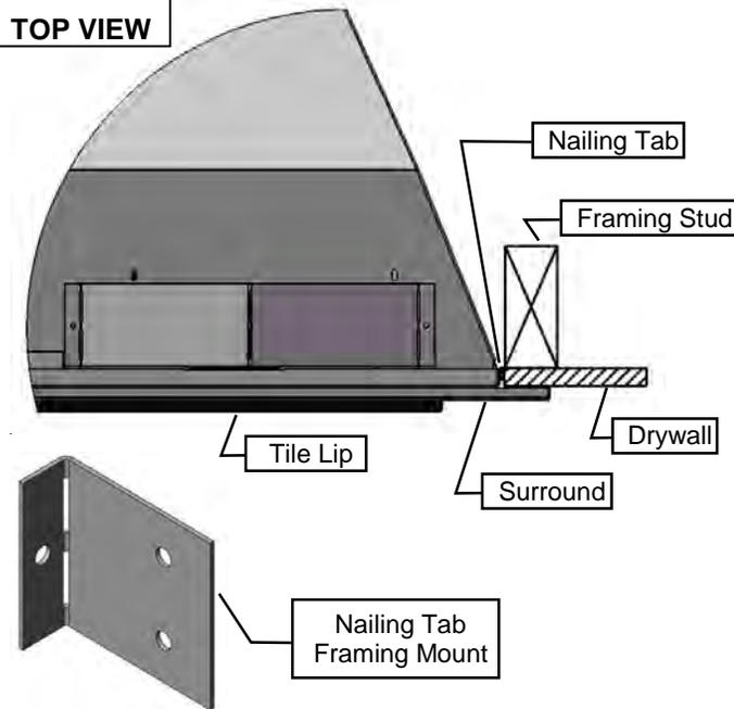
**Framing Flush with Face of Fireplace** -Fireplace to be covered with Non-Combustibles (e.g. Concrete Board) for Flat Wall appearance. **NOTE: 1/2" MUST BE ADDED TO FRAMING DEPTH OF UNIT. USE THIS METHOD FOR ZCVRB3622 SURROUNDS.**
