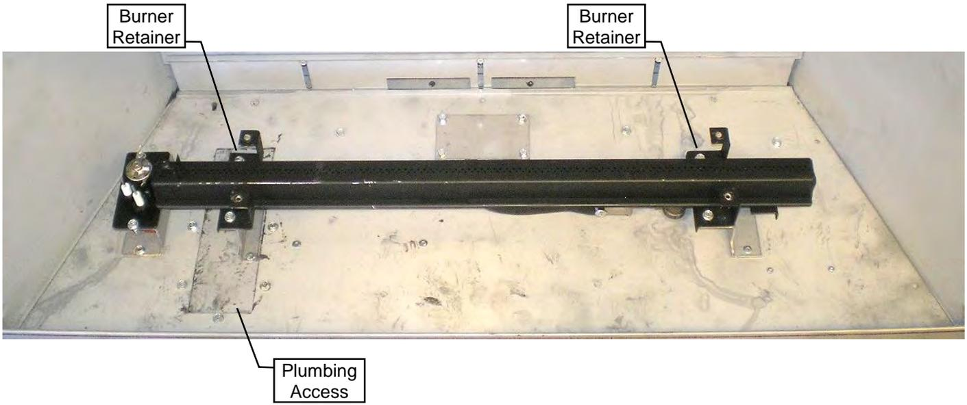
1. Remove four [4] screws holding down the false bottom. Remove the four [4] screws holding down the burner tube assembly.
