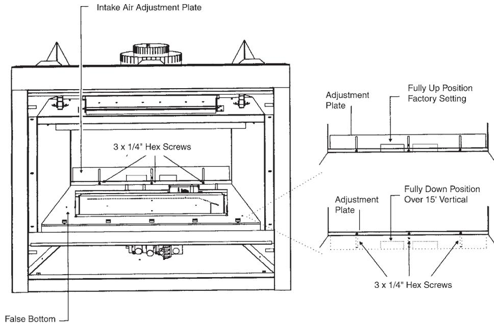
NOTE: Unit comes preset for short horizontal or vertical venting under a 15 feet run.
