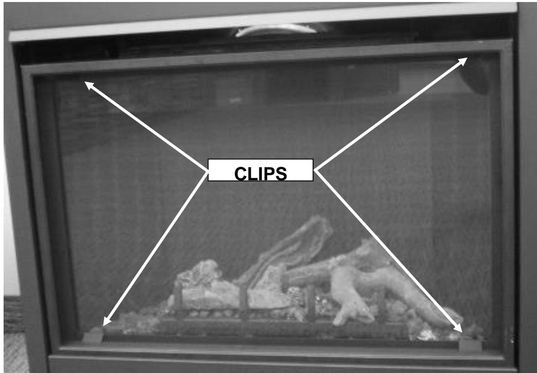
**To install screens** hook bottom clip onto glass door frame, then press down and push upper clip under top glass door frame, then release. Clip will hook onto frame.
