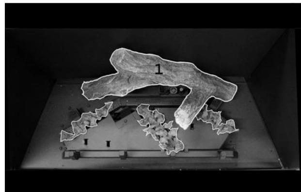
STEP 1: Place Log #1 onto the rear burner pan sliding it left until it stops against the right burner mount.
