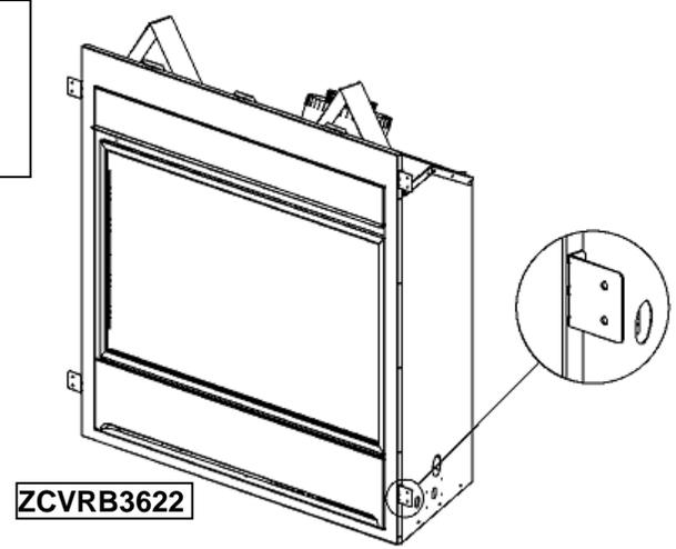
These Nailing Tabs can be used in two ways:
