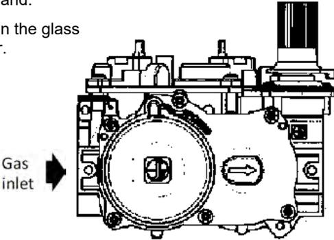
6. Turn manual shutoff valve clockwise ↻ to off (Located behind the access panel).
