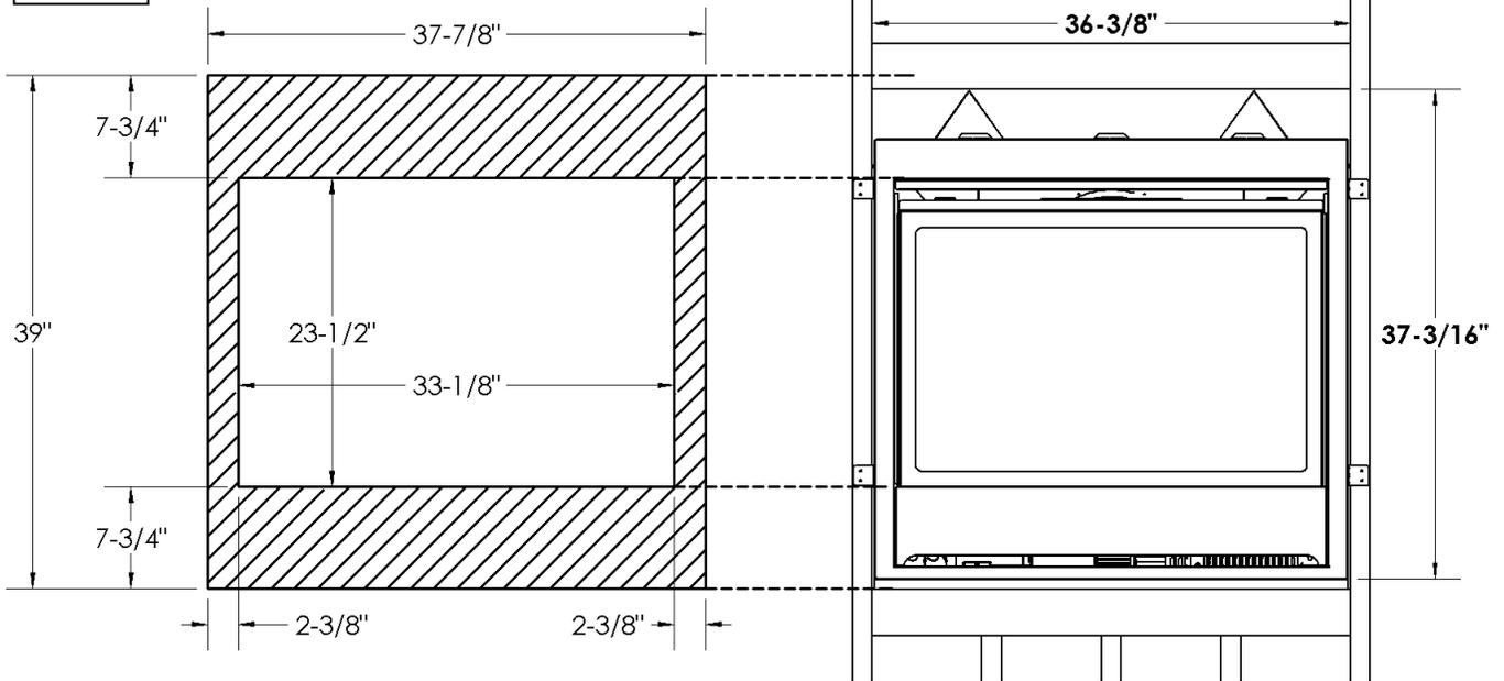
**Note:** Do not drive excessively long screws into the face of the unit as internal parts may be damaged.
