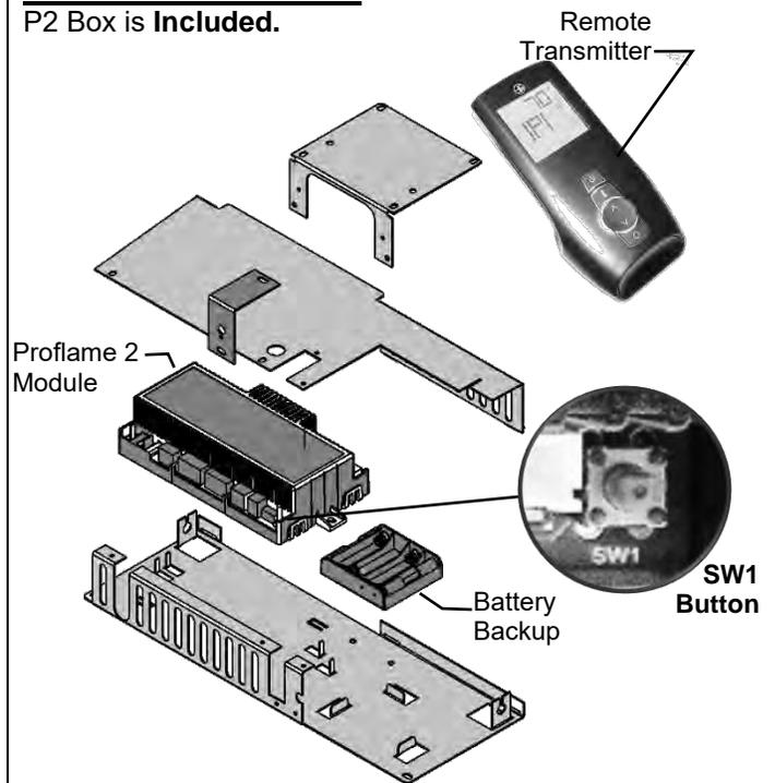
If Lower Panel has been covered, batteries may be changed through the Access Area, but burner pan must be removed to service or replace components (See **Burner Pan Removal** section of manual).
