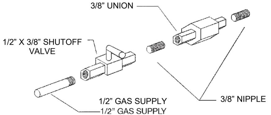
5. For natural gas, a minimum of 3/8" iron pipe with gas minimum pressure of 4.5" w.c. must be used for supply from the gas meter. Consult with the local gas utility if any questions arise concerning pipe sizes.
