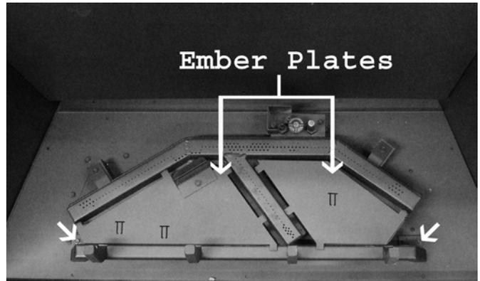
**Step 1:** Remove the grate bar by removing the 2 screws located on the left and right side of the grate bar as illustrated. Remove the 2 ember plates once the grate bar is removed. **The 2 screws removed must be re-installed once the grate bar is removed.**
