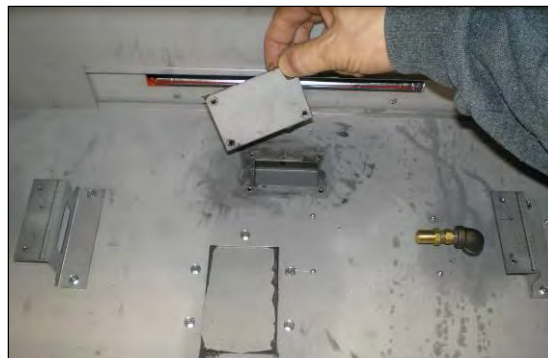
STEP 1: Remove false bottom to expose burner tube. Remove burner tube and cover plate as above. Remove old sealant from opening.
