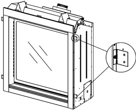
[Qty]2 Nailing Tabs are located on each side of the front frame.
