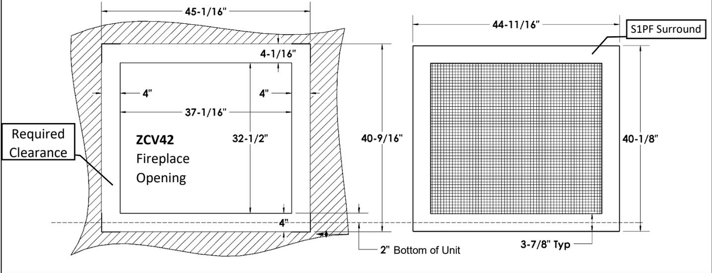
**ZCV39 / ZCV42 Basic Finishing 3: Concrete Board Behind S2PF Surround (3/4" Maximum Total Thickness)**
