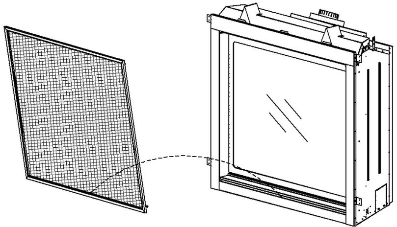
Place hook at bottom of screen onto frame of fireplace below Access Panel.
