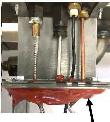
**NOTE:** Pilot connections through Burner Pan must be sealed with **Red Silicone**.
