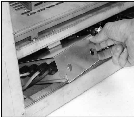
**NOTE:** Fireplace glass door must be removed to Install or remove Power Vent Control Module.
