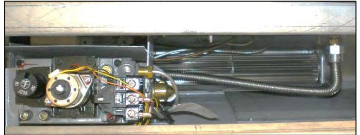
**NOTE: Do not allow cords or wires to come into contact with the firebox or the underside of the burner pan.**
