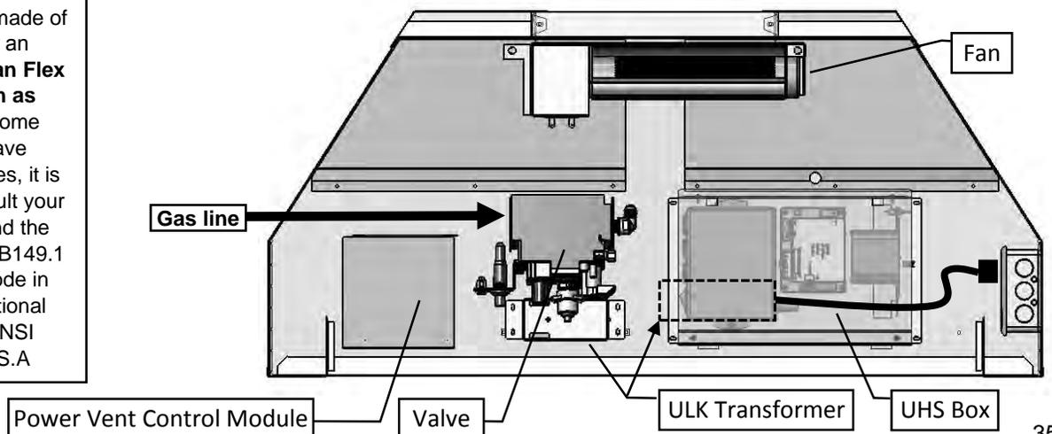
The fan can be installed through the side of the fireplace.
