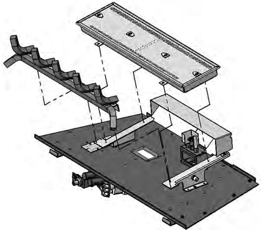
**Removal:** Remove Log Holder. Remove fourteen [14] screws around edge of Burner Pan. Carefully work the burner pan loose & lift the assembly upward to remove it from the firebox cavity.
