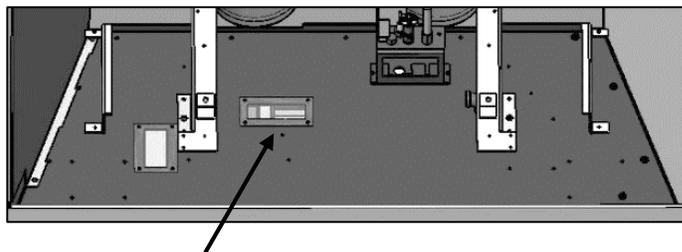
**STEP 1:** Remove Burner (See Burner Removal Section). **Remove Cover Plate.** Remove old sealant.
