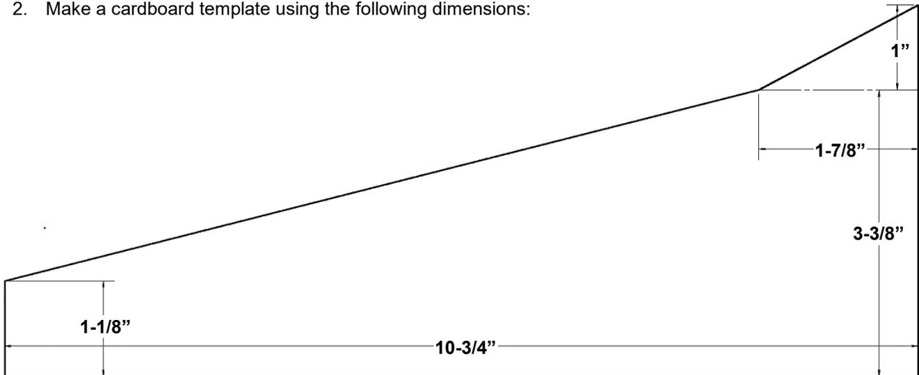
3. Use this template to mark and cut the bottom of the side liners.
