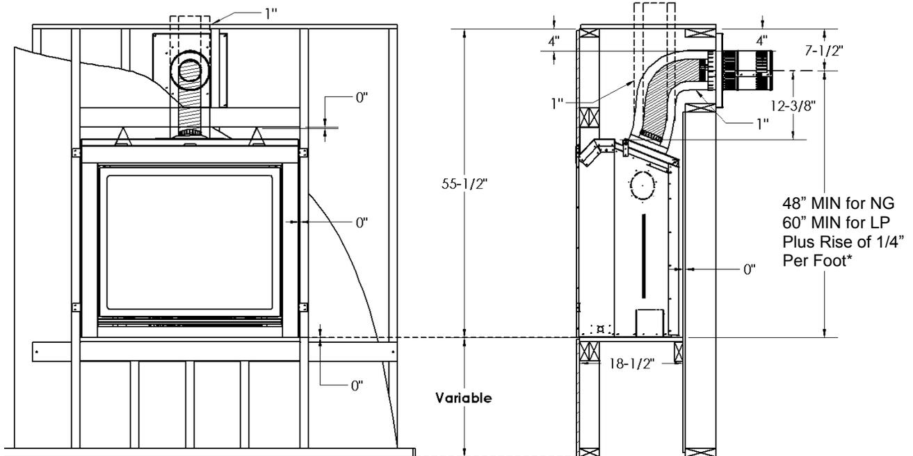
\*Note: If appliance is installed directly on carpeting or other combustible material other than wood flooring, a metal or wood panel extending the full width and depth of the appliance must be used. Carpet may extend 1 inch above the floor of the appliance.
