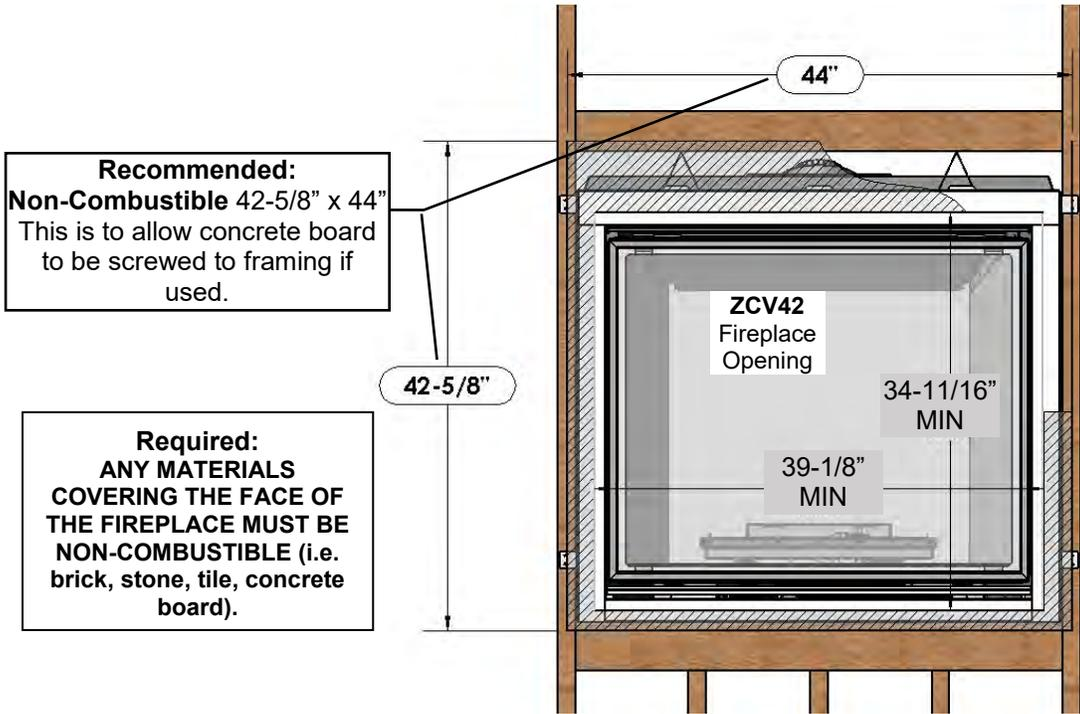
**Note:** Do not drive excessively long screws into the face of the unit as internal parts may be damaged.
