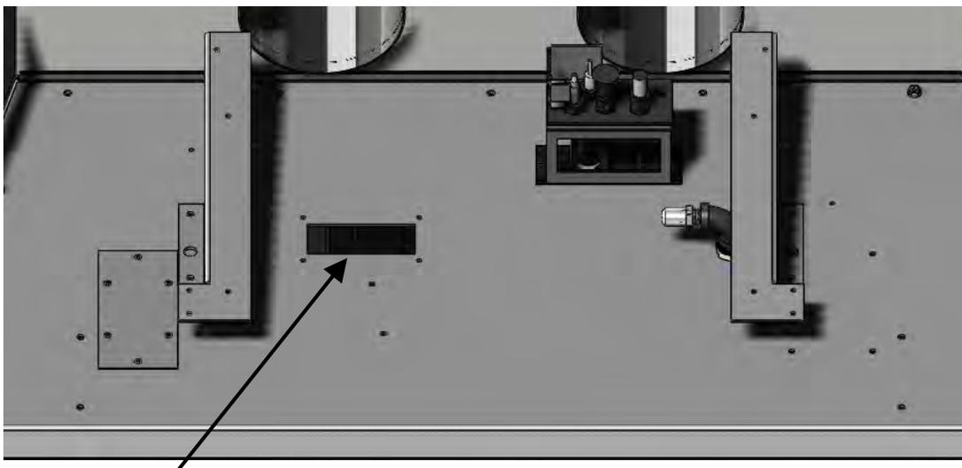
**STEP 2:** Insert Lamp Wires through access hole in firebox. **Apply New Sealant (Mill-Pac).** Secure Lamp Plate with screws.
