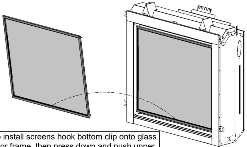
To install screens hook bottom clip onto glass door frame, then press down and push upper clip under top glass door frame, then release. Clip will hook onto frame.
