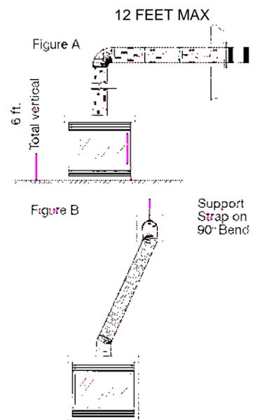
For Propane Horizontal installations the venting must be an additional one foot above the minimum vertical rise off the flue before going horizontal.
