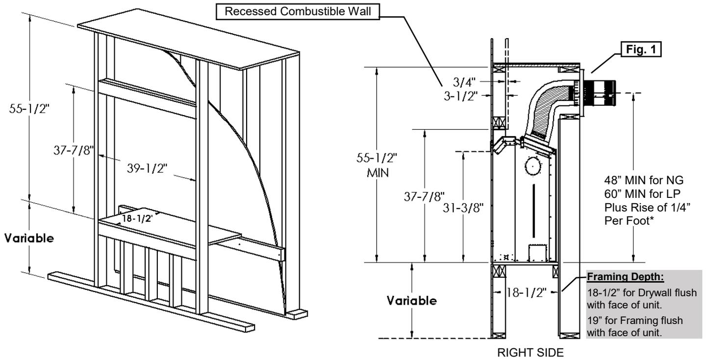
**\*For Propane Horizontal installations the venting must be an additional one foot above the minimum vertical rise off the flue before going horizontal.**
