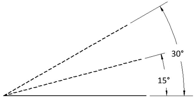
2. Engage door in lower latches at an angle of between 15 and 30 degrees.
