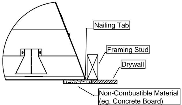
**Nailing Tabs Must Be Rotated 180° And Folded Back Onto Framing Stud.**
