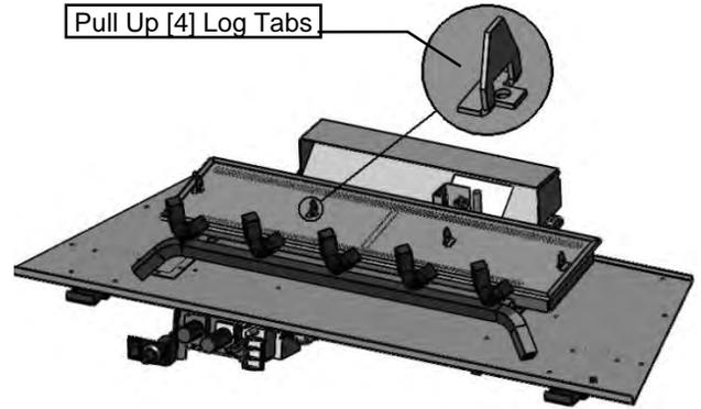
Pull up [4] Log Tabs on Burner. Match with Holes in Logs 4 & 5.
