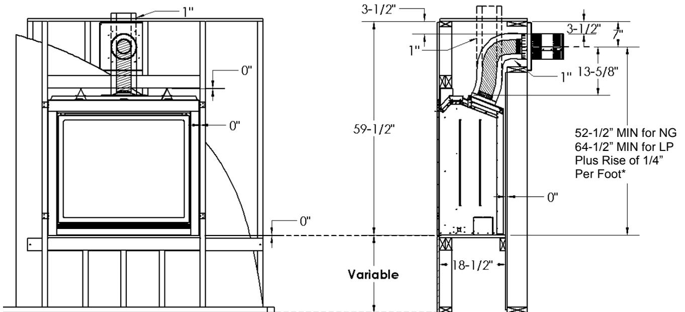
\*Note: If appliance is installed directly on carpeting or other combustible material other than wood flooring, a metal or wood panel extending the full width and depth of the appliance must be used. Carpet may extend 1 inch above the floor of the appliance.
