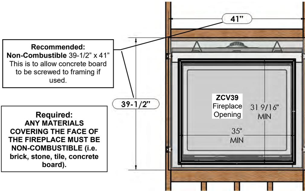
**Note:** Do not drive excessively long screws into the face of the unit as internal parts may be damaged.
