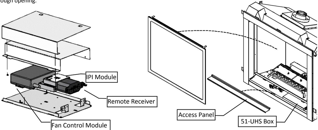
51-UHS can be inserted & removed from beneath fireplace through access panel opening (Remove glass door first).
