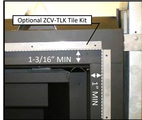
**Step 3:** Concrete Board with optional Tile Lip shown below.
