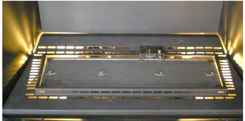
Glass may be used to cover perforations in false bottom
