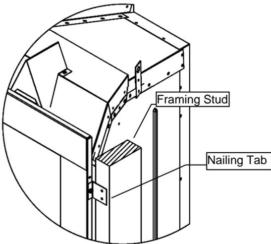
**Framing Flush with Face of Fireplace -**Fireplace to be covered with Non-Combustibles (e.g. Concrete Board) for **Flat Wall** appearance.
