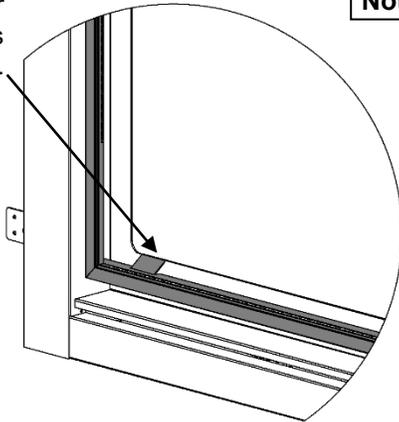
Press down and push Upper Clip under top glass door frame.
