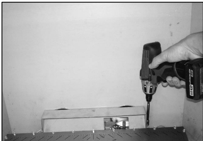
Step One: Remove Log Holder.
