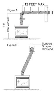
Two snorkel terminations are available if a vertical rise is necessary on the exterior side of a building:
