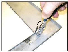
Place surround face down on protected surface. Bend Top Hook and Lower Mount Tab up 90° from surface.
