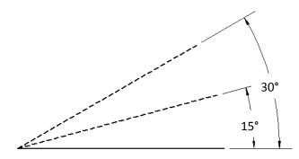
2. Engage door in lower latches at an angle of between 15 and 30 degrees.
