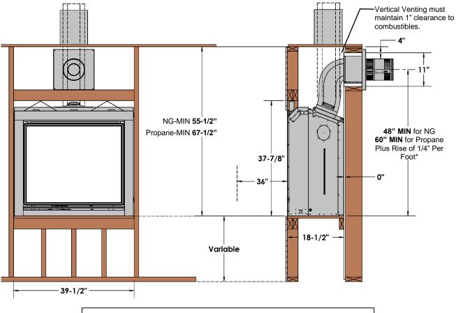
\*Note: If appliance is installed directly on carpeting or other combustible material other than wood flooring, a metal or wood panel extending the full width and depth of the appliance must be used. Carpet may extend 1 inch above the floor of the appliance.
