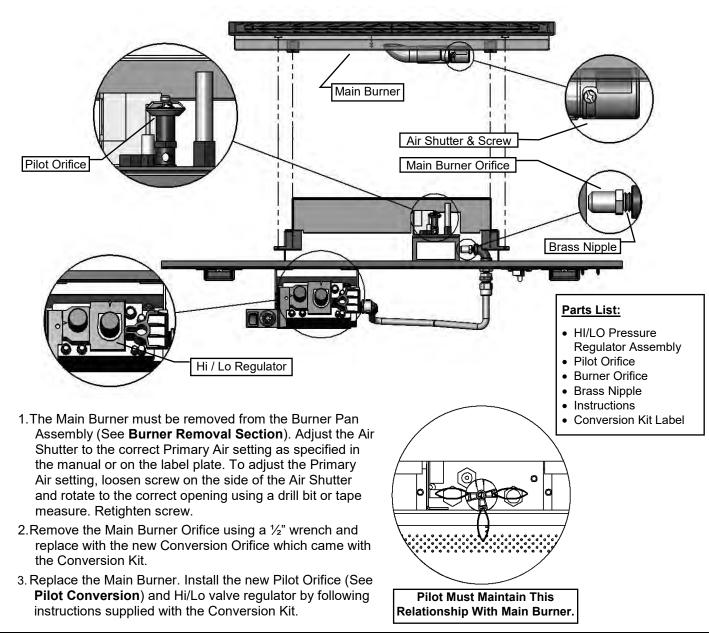
Refer to "Gas Specifications Chart" for inlet pressures and input ratings. Clock meter to verify input rate. Place conversion label as close to converted gas control as possible. Refer to lighting instructions to verify the normal operating sequence of the ignition system.
