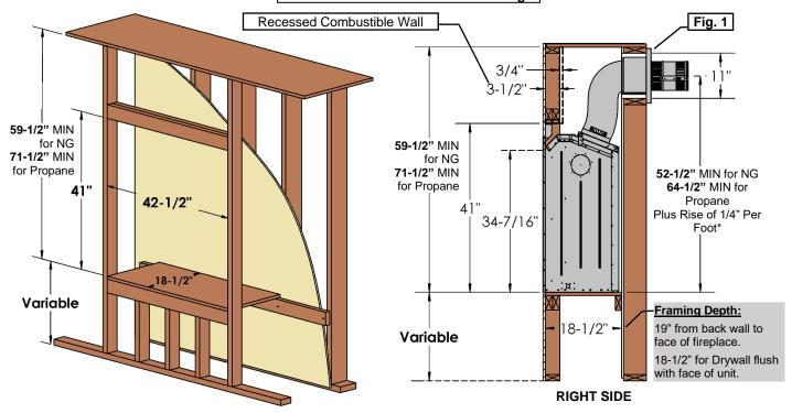
\*For Propane Horizontal installations the venting must be an additional one foot above the minimum vertical rise off the flue before going horizontal.
