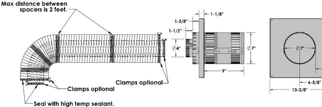
Secure with 4 screws per pipe joint.
