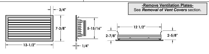
Installation: Insert Grills into openings and fasten to framing with a wood screw at each end.
