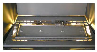
Glass may be used to cover perforations in false bottom
