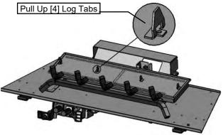
Pull up [4] Log Tabs on Burner. Match with Holes in Logs 4 & 5.
