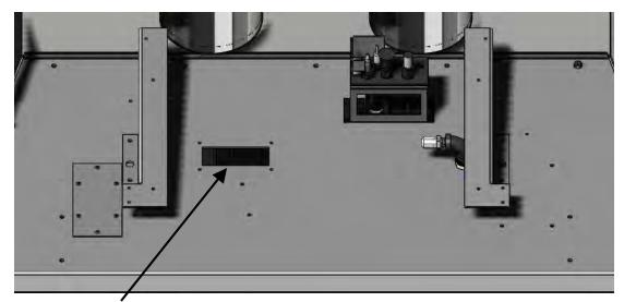
STEP 2: Insert Lamp Wires through access hole in firebox. Apply New Sealant (Mill-Pac). Secure Lamp Plate with screws.
