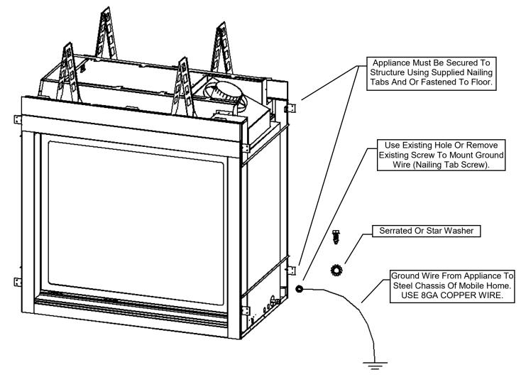
THE VENTED GAS FIREPLACE HEATERS (ANSI Z21.88) IN THIS MANUAL MAY BE INSTALLED IN MANUFACTURED (MOBILE) HOMES AFTER FIRST SALE IN THE USA.
