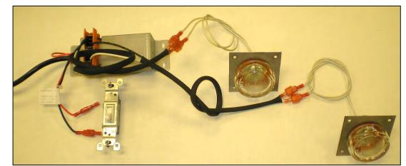
**STEP 2**: Connect lamp wires to jacketed transformer leads. Connect switch wires to black and red wires at transformer, or plug black and red transformer wires together if 120V receptacle will be switch controlled.
