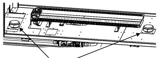
STEP 1: Remove cover plates and install lamps in firebox. Seal with fresh sealant (Mill-Pac).
