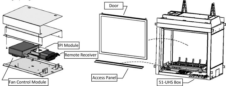
51-UHS can be inserted & removed from beneath fireplace through access panel opening (Remove glass door first).
