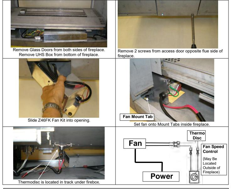
NOTE: Do not allow cords or wires to come into contact with the firebox or the underside of the burner pan.
