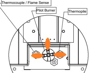
It is recommended to turn on the unit at least once a month and inspect the flame pattern to ensure there are no problems with the burner tube (Flame should appear similar to the above picture).
