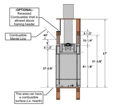
Any materials covering the face of the fireplace **MUST** be non-combustible (i.e. brick stone, tile, concrete board).
