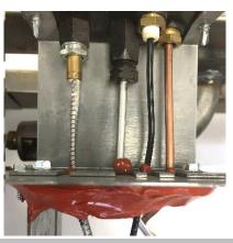
**NOTE:** Pilot connections through Burner Pan must be sealed with **Red Silicone**.
