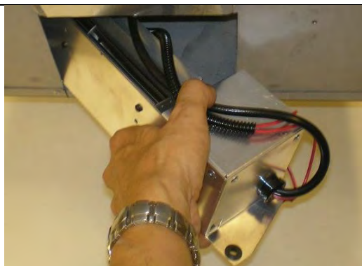
Slide Z46FK Fan Kit into opening.
