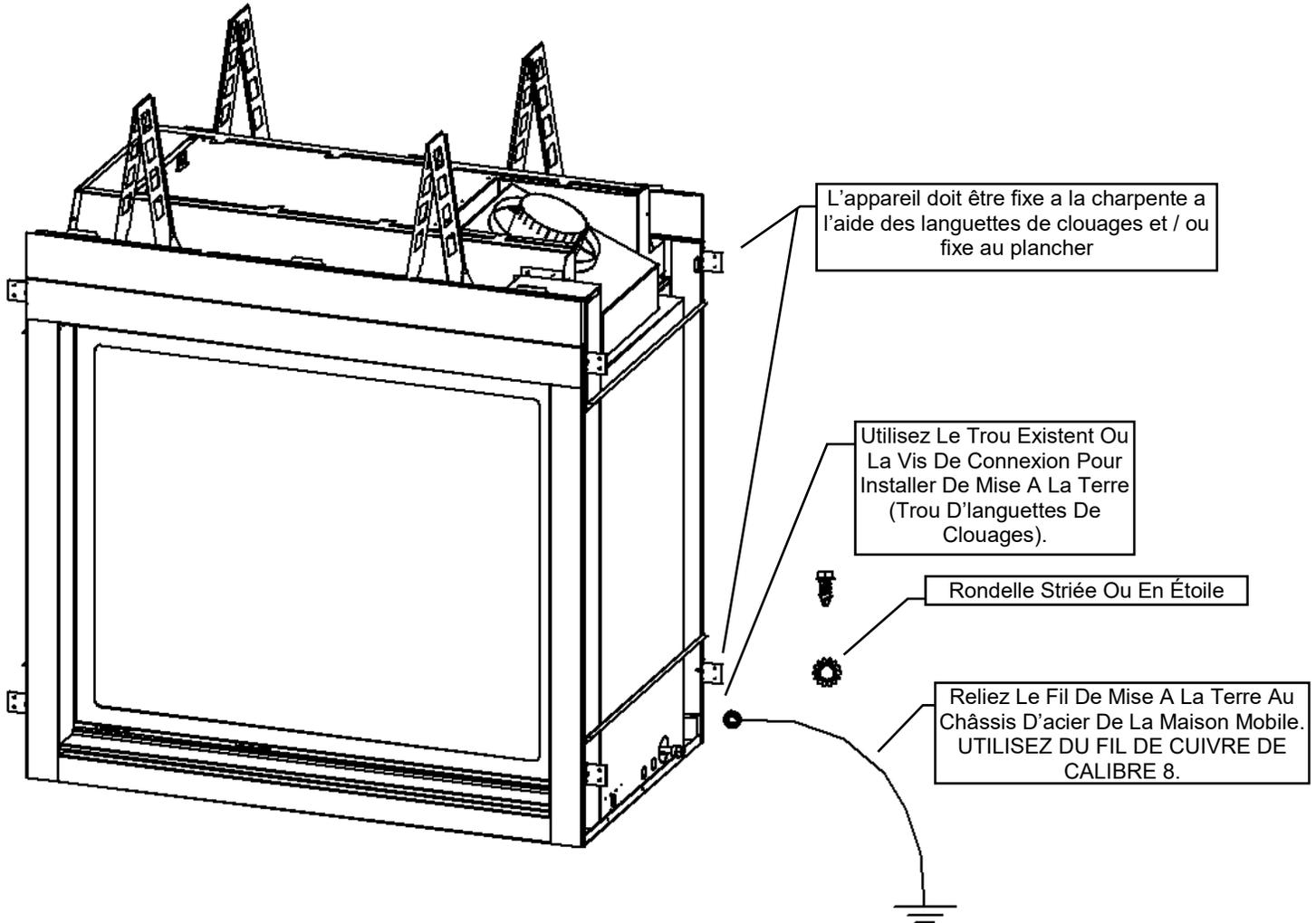
LES CHAUFFAGES À FOYER À GAZ VENTILÉ (ANSI Z21.88) DANS CE MANUEL, PEUT ÊTRE INSTALLÉ DANS FABRIQUÉS (MOBILES) LA PREMIÈRE VENTE APRÈS DANS LE ÉTATS-UNIS.
