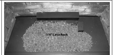
**Step #1-** Place 1/4" Lava Rock Onto and around Burner Pan as shown, Do Not place lava rock into pilot shield assembly area.
