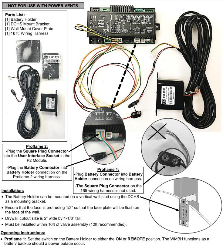
• **Proflame 2:** Set the switch on the Battery Holder to the **REMOTE** position. **NOTE:** If the switch on the Battery Holder is set to **ON**, the remote control will be disabled. The WMBH functions as a battery backup should a power outage occur. Refer to the manual that accompanies the Battery Holder for further instructions.
