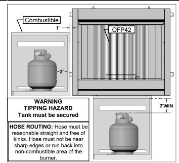
There shall be a minimum clearance of 2 in (50.8 mm) between the floor of the non-disposable LP-gas cylinder enclosure and the ground.
