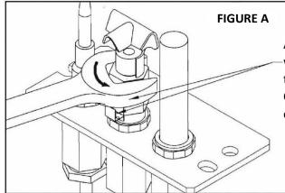
Avoid contacting Orifice Strip with end wrench. Failure to do this can cause distortion of the Orifice Strip when loosening or tightening.
