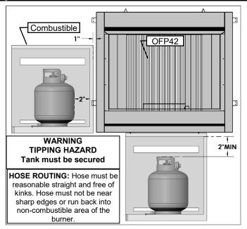
There shall be a minimum clearance of 2 in (50.8 mm) between the floor of the non-disposable LP-gas cylinder enclosure and the ground.
