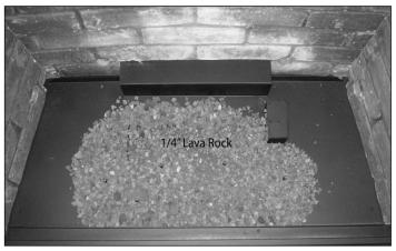
**Step #1** – Place 1/4" Lava Rock onto and around outer Perimeter of the Pan Burner as shown. Leave the Log Placement Pins exposed.
