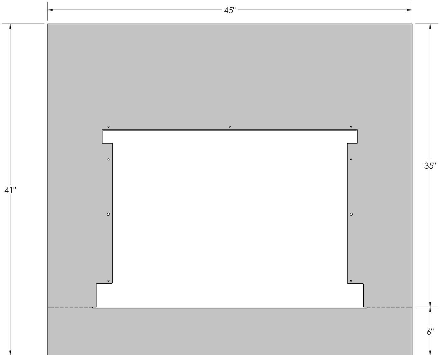
Cut Surround at dotted line shown above to make the bottom flush with the fireplace bottom.
