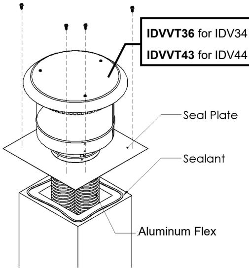
1. Before attaching the flex vents to the termination, you will have to determine how the cap will be attached to the existing chimney crown, clay lined chimney or wood stove vent pipe. The Seal Plate of the termination may be cut, notched and formed to make a good seal to the existing vent or be left flat.
