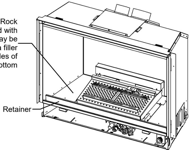
**Setup:** Place Glass Embers over tray and on firebox bottom (left and right). **Do not cover pilot shield area.** See Glass Ember Installation page for further details.
