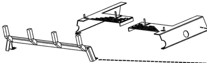
**Preparation:** Remove Grate Bar and replace screws. Remove Ember Plates. Do not remove existing Pilot Shield.
