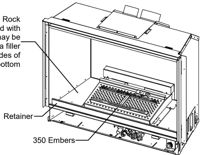
**Setup:** Place a thin layer of 350 Embers onto burner tube. Place Lava Rock over tray and on firebox bottom (left and right). **Do not cover pilot shield area.** See Glass Ember Installation page for further details.
