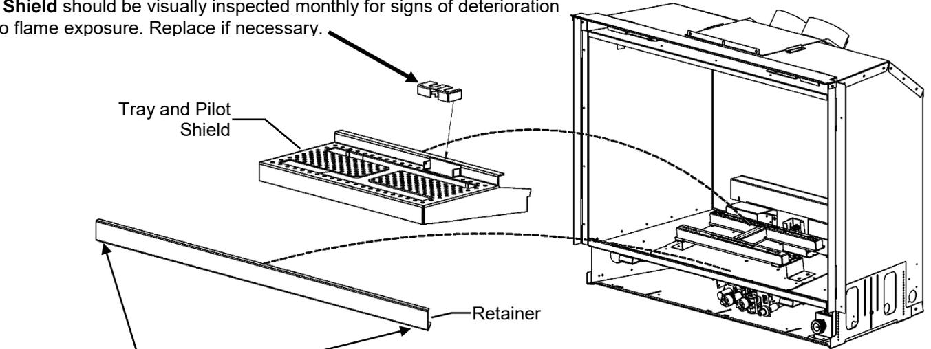
Use existing screws to attach Glass Retainer.
