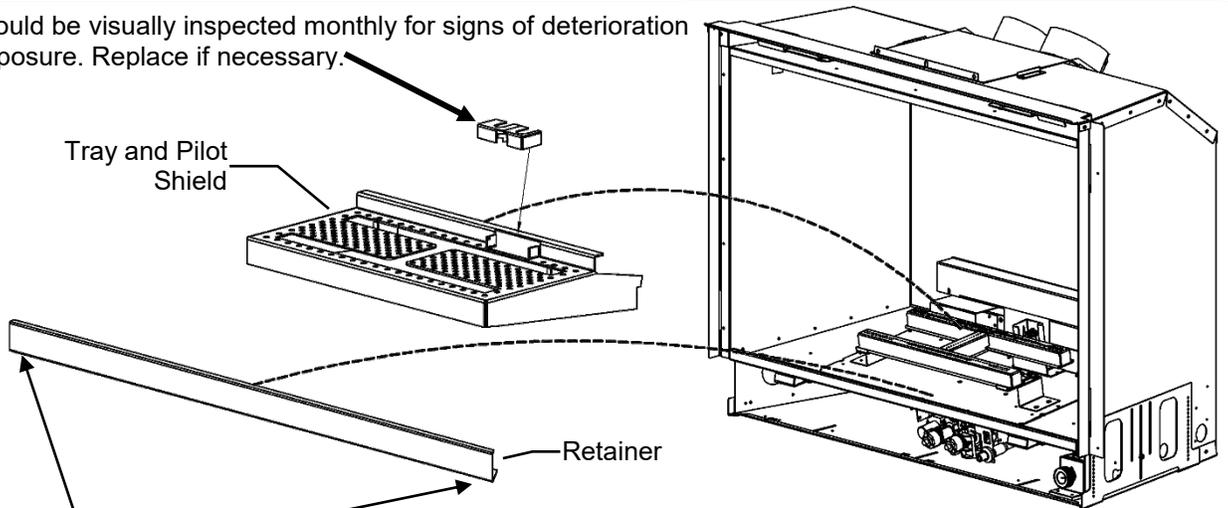
Use existing screws in firebox bottom to attach Retainer.
