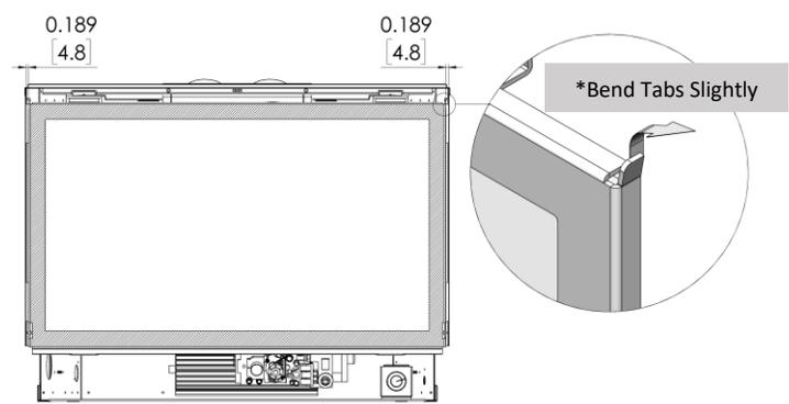
**\*RECOMMEND:** Slightly bend the two [2] upper door tabs (~10°) as shown above to help ease installation of Safety Screen. DO NOT OVERBEND.
