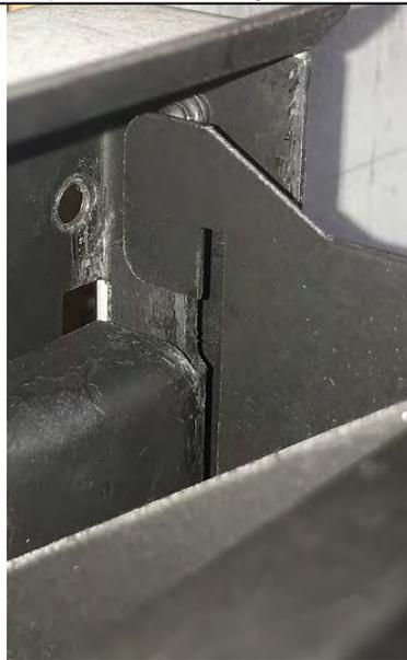
**3: Lower Screen.** Watch both sides to ensure that Top Hooks engage properly.
