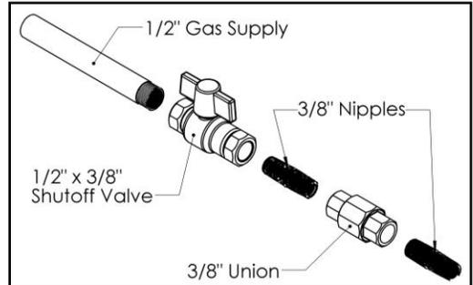
Shutoff valves installed in tubing systems shall be rigidly and securely supported independently of the tubing.
