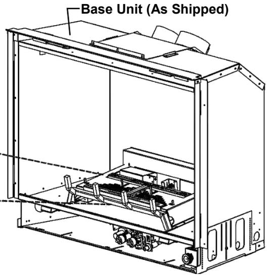
**Preparation:** Remove Grate Bar and replace screws. Remove Ember Plates. Do not remove existing Pilot Shield.
