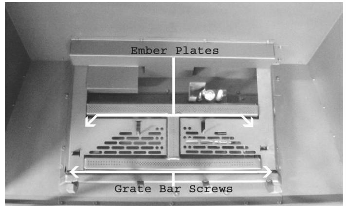
Remove the ember plates and the grate bar by removing the 2 left and right screws on the grate bar.
