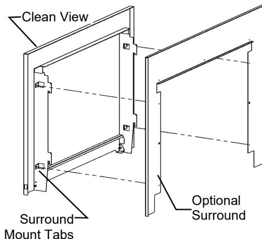
**SECTION 2: Clean View Mount Slots** are located beside the Safety Screen Frame on the Fireplace. Insert the [4] Clean View Mount Hooks into the **Clean View Mount Slots** and lower the Clean View into place.
