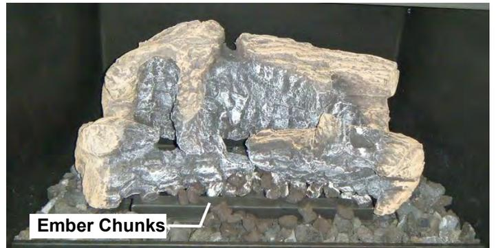
A bag of **Ember Chunks** is supplied with the appliance. It is very important that these chunks are placed onto the front burner and log mounting pan as shown in the picture. Spread the Ember Chunks out no more than one layer deep.
