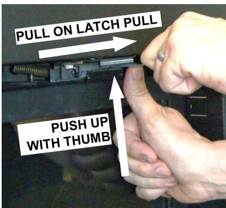
1. Disengage Top Latches by pulling on Latch Pull with one hand and pushing up on Latch Pull with the thumb of your other hand (See Photos to left).
