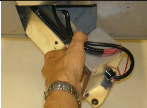
Slide Z46FK Fan Kit into opening.
