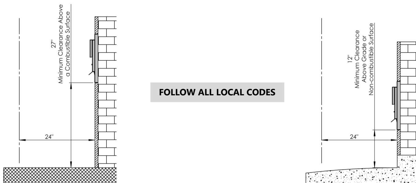
Figure 1 - Exterior discharge clearances.
