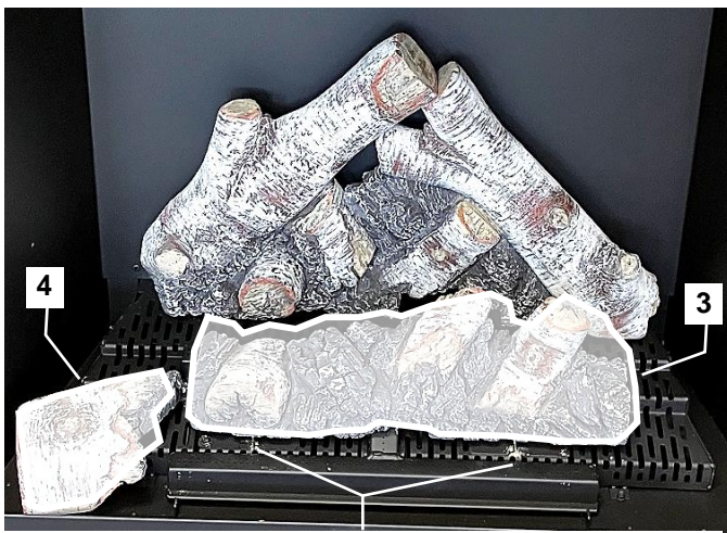
Set Log 3 onto center of Burner and pull forward up to Log Tabs. Place Log 4 at front left side of Firebox.
