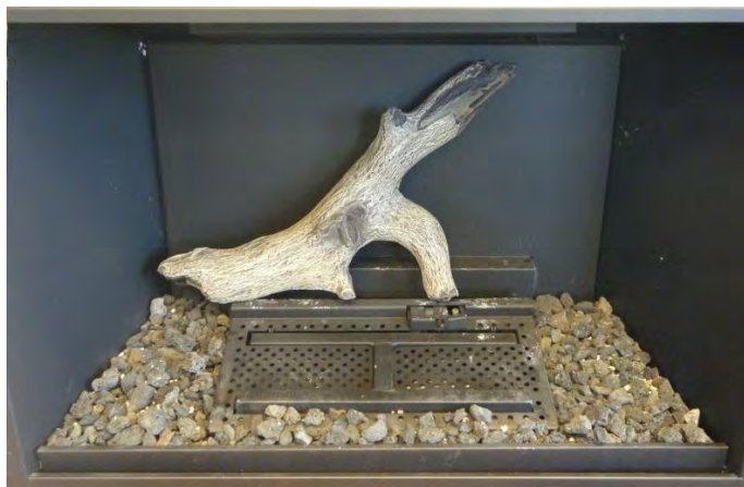
STEP 1: Fill bottom of firebox around tray with Lava Rock and place LOG 1 against back wall as shown.
