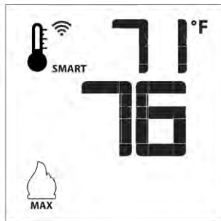
Fig. 11: Smart flame function
