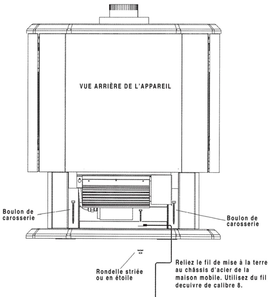
**LES MODÈLES FDV350N ET FDV350LP PEUVENT ÊTRE INSTALLÉS DANS DES MAISONS USINÉES (MOBILES) APRÈS LA PREMIÈRE VENTE. LES MODÈLES CONVERTIS UTILISANT LE CONVERTISSEUR TYPE B NE PEUVENT PAS ÊTRE INSTALLÉS DANS DES MAISONS USINÉES (MOBILES).**
