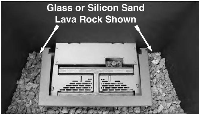
STEP 4: Fill around the rock platform with lava rock. Do not place any lava rock on the burner. Sprinkle vermiculite over top of the lava rock.
