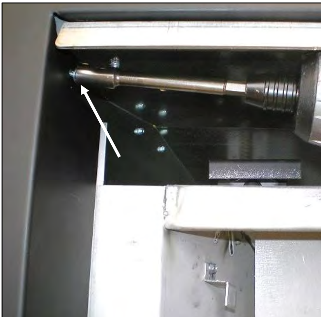
Step 3 (illustrated): Install screws in top corners.
