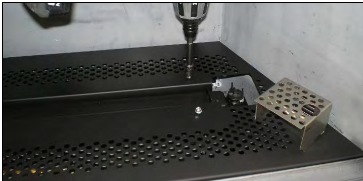
Remove False Bottom, Pilot Cover, and Upper Baffle.
