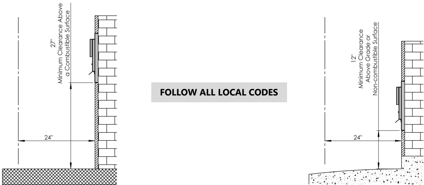
Figure 1 - Exterior discharge clearances.
