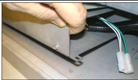
2. Lift UHS Box out of Unit
