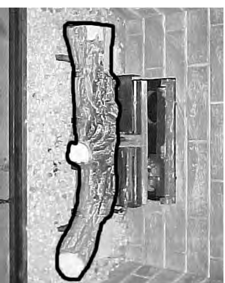
Step (3) Place front log by positioning the notches on the underside of the front log with the grate bars and pull forward.
