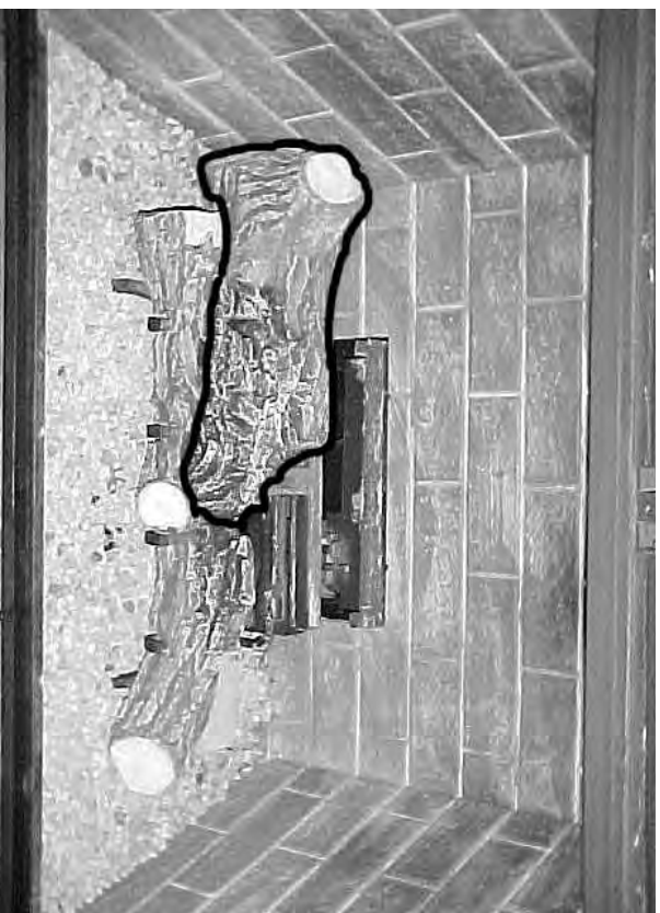
Step (4) Place left front log by positioning the slot (located on the bottom of log) with log retainer tab and lower into position.
