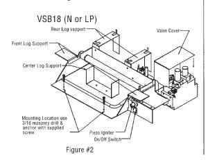
Wounting Location use 3/16 masonry drill & anchor with supplied screw.
