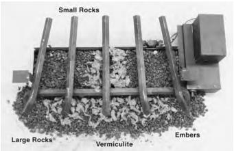
Place silica sand (NG only) or 1/4" small rock (LP only) inside and in front of burner pan. Place 1" large rock inside, in front, and around the sides of the pan. Place rock wool inside the middle of the pan and in front of the grate bar.. Sprinkle vermiculite over top of lava rock and rock wool.
