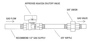
For the state of Massachusetts a **T-handle gas shut- off valve** must be used on a gas appliance. This Thandle gas shut-off valve must be listed and approved
