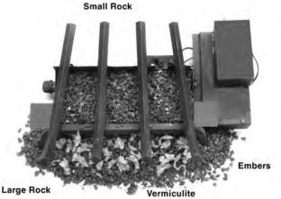
Place silica sand (NG only) or 1/4" small rock (LP only) inside and in front of burner pan. Place 1" large rock inside, in front, and around the sides of the pan. Place rock wool in front of the grate bar. Sprinkle vermiculite over top of lava rock and rock wool.
