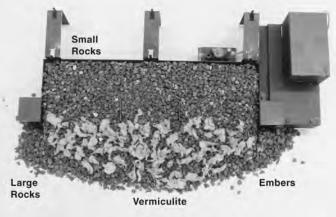
Place silica sand (NG only) or 1/4" small rock (LP only) inside and in front of burner pan. Place 1" large rock inside, in front, and around the sides of the pan. Place rock wool in front of center log support as shown. Sprinkle vermiculite over top of lava rock and rock wool.
