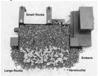
Place silica sand (NG only) or 1/4" small rock (LP only) inside and in front of burner pan. Place 1" large rock inside, in front, and around the sides of the pan. Place rock wool in front of center log support as shown. Sprinkle vermiculite over top of lava rock and rock wool.
