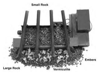
Place silica sand (NG only) or 1/4" small rock (LP only) inside and in front of burner pan. Place 1" large rock inside, in front, and around the sides of the pan. Place rock wool in front of the grate bar. Sprinkle vermiculite over top of lava rock and rock wool.
