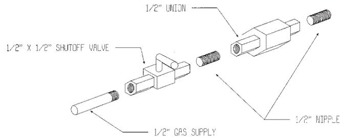
**Important:** Always check for gas leaks with a soap and water solution. Do not use open flame for leak testing.
