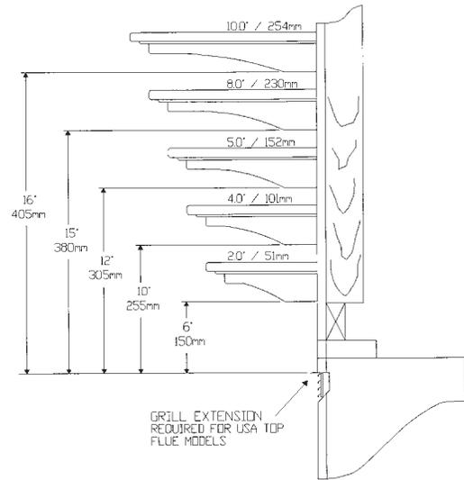
**Warning:** Combustible objects must not be placed on a non-combustible mantle unless the non-combustible mantle meets the minimum height and width requirements for a combustible mantle.
