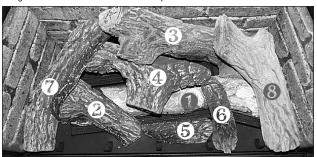
**STEP 8:** Place a small amount of glowing ember material (a) onto the front burner tube ends. (Too much ember material causes a blue flame.) (When placing embers onto burner, leave an air space between the log and the embers; this will help produce a yellow flame in these areas.) Place rocks (n) onto false bottom only. Do not place rocks onto burner tubes.
