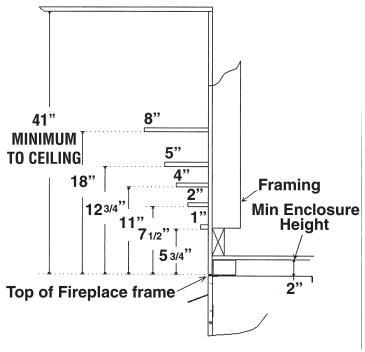
FIGURE 7 – Minimum Clearances - Top and Sides of Room Heater to Ceiling and Walls.
