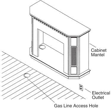
FIGURE 9 – Installing Cabinet Mantel
