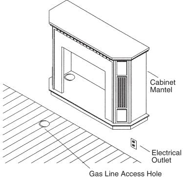
FIGURE 9 – Installing Cabinet Mantel
