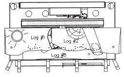
STEP 4 Position log #4 onto rear log holder and pull up to logs 1 and 2.
