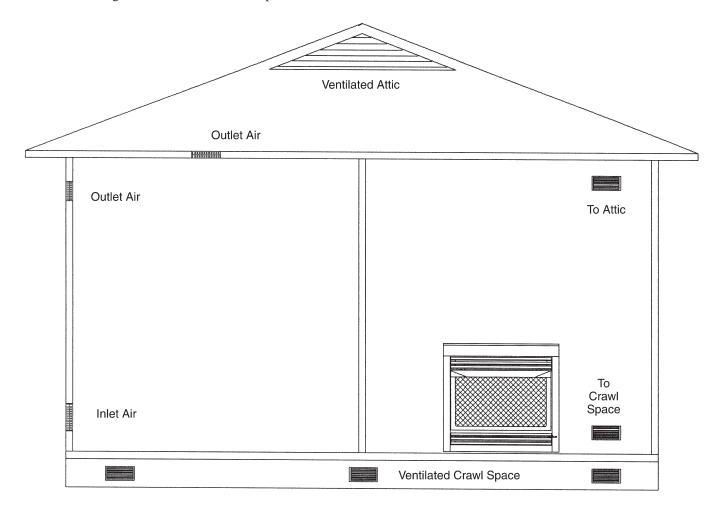
FIGURE 6 - Ventilation Air from Outdoors
