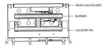
STEP 1 Locate hole on underside of log and place log over burner and Locator Pin and lower into position.
