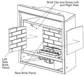
FIGURE 13 - Installing Brick Panels
