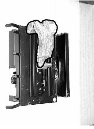
**Step (2)** Locate hole on the underside of Log C. Place log over front burner and locator pin then lower into position (as illustrated).
