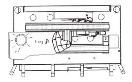
STEP 2 Locate hole on underside of  $\log$  and place  $\log$  over burner and Locator  $\Pr$  and  $\log$  into position.
