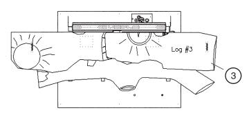
STEP #4. Place rear log onto rear log holder and pull up to left and right front logs.
