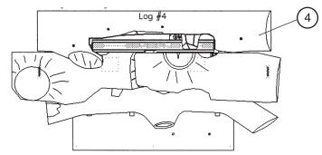
STEP #5 & 6. Line up holes on crossover logs with locator pins on rear log #4 and lower into position.
