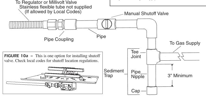
FIGURE 10, 10a - Installing gas line and manual
