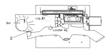
STEP #3. Locate right front Log by positioning slot on bottom of log with Tab on support bracket and lower into position.
