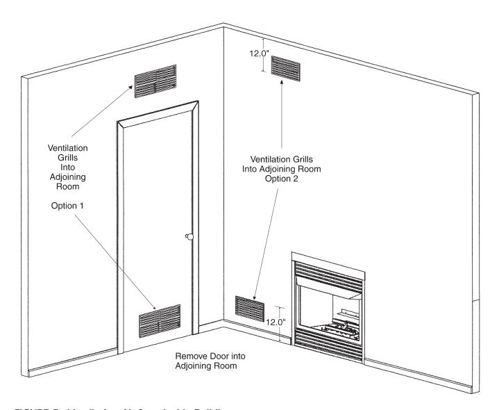
FIGURE 5 - Ventilation Air from Inside Building
